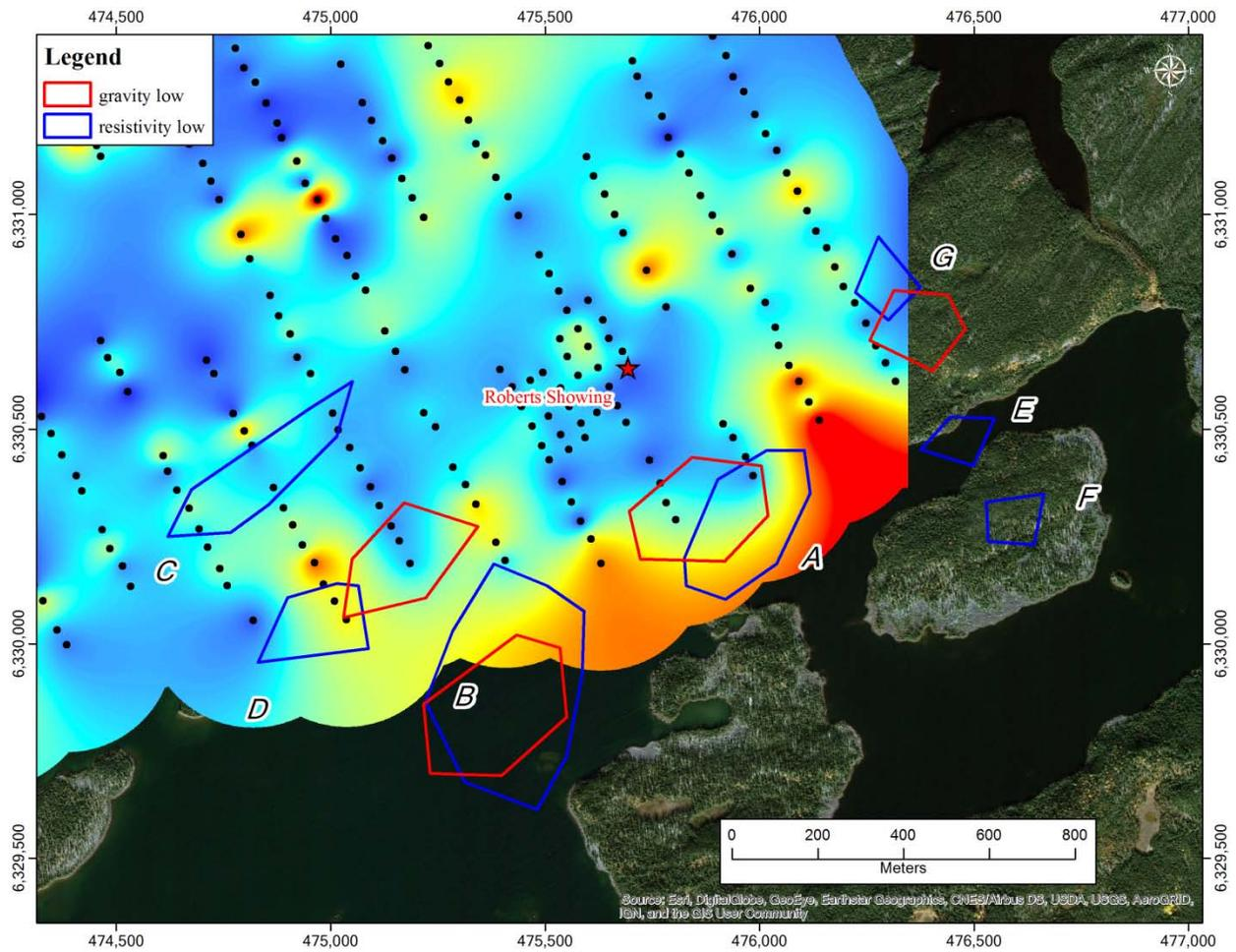
**Figure 9. Radon, Resistivity and Gravity Anomalies**
