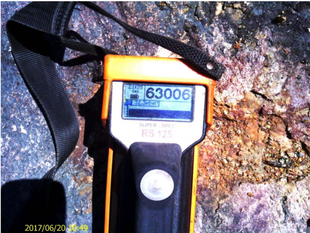
**Photo 2. Spectrometer Reading at the Roberts' Showing (in cps)**
